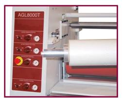
Cantilevered Material Shafts
