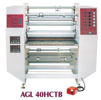
Heated chrome top nip roll with heated silicone bottom nip roll. Top and bottom let-off stations and release liner windup stations. Dual automatic transducer tension control and segmented
