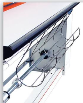
**RTS Brake** - (Repeatable Tension System Brake) - Adjusting film tension for prints that curl up or
