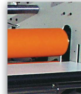
This feature makes sure you never have to worry about hot spots that will damage your prints. Other types of temperature sensors are fooled when you run cooling fans or when the rollers are stopped, causing them to over heat sending the temperature higher. This over heating can cause de-laminating of the silicone coated rollers.
