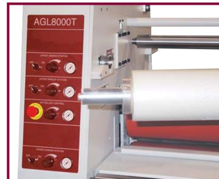
Cantilevered Material Shafts
