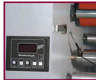
Proportional Electronic Tension Transducer for Automatic Web Tension Control
