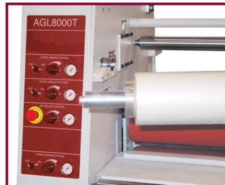
Cantilevered Material Shafts
