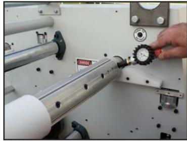
The outside diameter of an air shaft is slightly less than the inside diameter of the core of laminating film that you want to load into the laminator. Once the core of material is in its proper location on the air shaft an inflation tool injects air into a bladder inside the air shaft where by expanding either lugs or leaves to grab the core of material.
