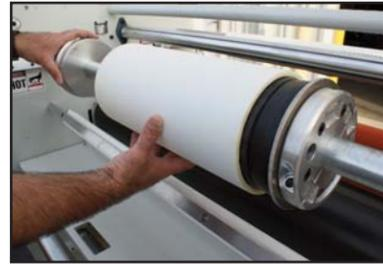
**Large Diameter Core Adaptors** – When you need to use a 6 inch core of material on your laminator, AGL's optional pneumatic core adaptors offer
