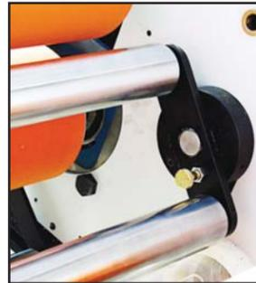
excessive brake tension that can cause post de-lamination. Stop running out (wasting) 5,10,15 feet of film just to get the film to lay flat. Start forming your film to the flat state your customer expects. Got up curl? Simply rotate the curl cam and its gone! The Curl Cam has a unique 360 degree rotation so you can make the changes you need without un-webbing your film!
