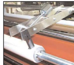
**Unwind Slitting** – is used to convert a wide roll of film on the unwind shaft to a smaller width web while laminating. The unused material remains on the roll core while the laminating material is introduced into the laminating process. The blade holder is a
