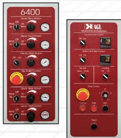
AGL 6400 Laminates and mounts a 62.0" wide maximum thermal or pressure sensitive film and features pneumatically actuated nip roller and pull roll assemblies. Main supply rolls are equipped with a pneumatic clutch/brake assembly. This feature allows precise and repeatable film tension control as well as bi-directional unwind/rewind capabilities.
