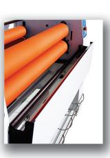
from the bottom supply shaft and never have to crouch under the table or get on your knees (a laborious task on other laminators). The Easy Web Feed Table also features a dual latch for secure docking, yet has an elegant single handle release making it a smooth and fast one handed operation. Another not so obvious, but strong, feature on the Easy Web Feed Table is the hidden film guide. When the table is in the "disengaged
