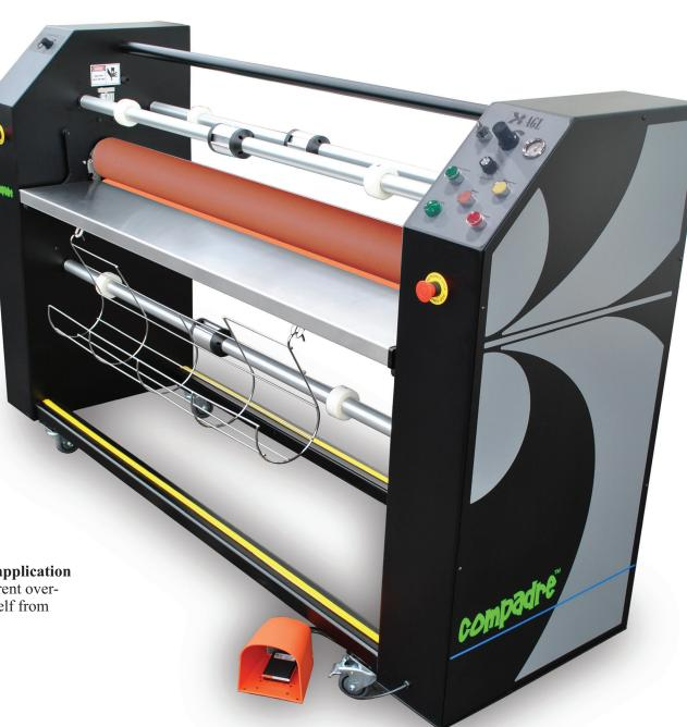
The Compadre is a laminator designed to satisfy the small to medium sign shop market. This laminator incorporates AGL's original nip roll design and configuration. The Compadre allows for more reliable print laminating and mounting at faster throughput speeds. It features a six inch diameter steel core covered with a high release non-crowned silicone covering. The top nip roll features preset heat assist for warming up pressure sensitive over-laminates to reduce or eliminate silvering.
